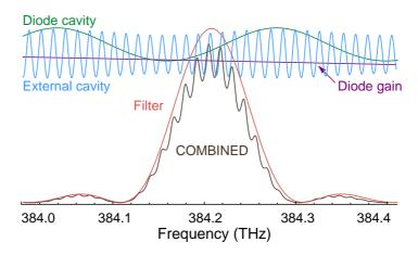
Figure 3.2: Schematic representation for the various frequency-dependent factors of an ECDL, adapted from Ref. [1], for wavelength  $\lambda = 780$  nm and external cavity length  $L_{\rm ext} = 15$  mm.
