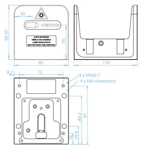
Figure A.2: Dimensions of previous generation LDL laser head.
