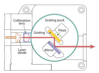
**Figure 1.3:** Cross-section of MOGLabs LDL Littrow laser, showing arrangement of laser diode, collimation lens, grating, piezoelectric transducer and fold mirror. The grating angle and hence wavelength is adjusted by rotating the central cylinder (the grating puck) which forms a rigid mount for grating and mirror.
