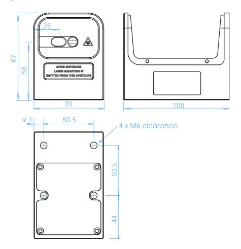
Figure A.1: Dimensions of compact LDL laser head.
