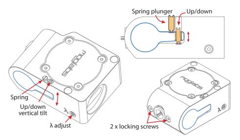
**Figure 4.4:** Sketch showing location of vertical alignment adjustments: a fine adjustment screw to push the laser diode beam upwards, and a spring plunger that pushes downwards.
