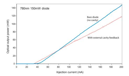
**Figure 2.1:** Sample laser diode power-current *PI* characteristic curves, with and without an external cavity. The external cavity feedback reduces the threshold current, and also the apparent power/current slope because the measured power with feedback is not the power from the bare diode, but the output beam reflected from the grating. The slope with feedback in this example is 75% of the bare diode output slope, consistent with the grating direct reflectivity.
