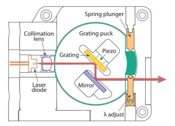
**Figure 3.1:** Cross-section sketch of the MOGLabs LDL, showing the cylindrical grating mount (puck), piezo-mounted grating, fold mirror, and wavelength adjustment. The grating mount can be rotated using the tangential  $\lambda$  fine adjustment screw. A counteracting spring-plunger should be released to allow rotation.
