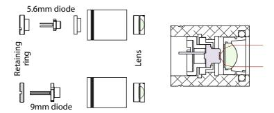
**Figure 4.1:** Lens tube assembly, showing diode, lens, and mounting hardware. The same tube can be used for 5.6 mm and 9 mm diodes.
