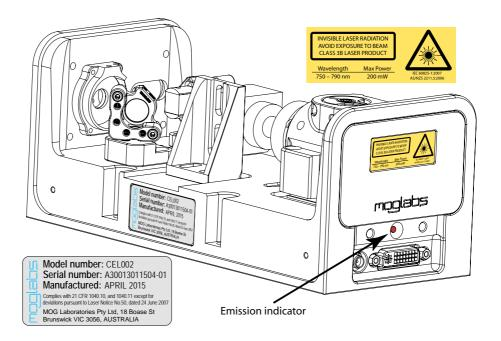
**Figure 3:** Schematic showing location of laser warning labels for the large-chassis CEF version of a MOGLabs laser.
