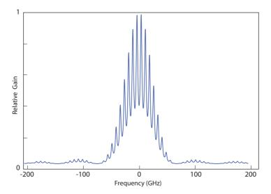
**Figure 3.3:** Combined gain for an external cavity diode laser, including the internal and external modes, the diode laser gain, and the filter response. The broad feature is the frequency selectivity of the filter, and the smaller peaks are the external cavity modes (see fig. 3.2). A small relative shift of the external cavity mode relative to the filter frequency will cause the laser to jump to another external cavity mode where the net gain is higher.
