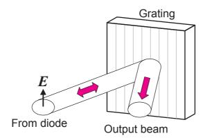
**Figure 4.3:** Orientation of the diode laser beam ellipse with respect to the diffraction grating.
