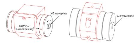
**Figure 4.7:** Two types of Faraday isolator. Each can be supplied with exit  $\lambda/2$  waveplate inside one end-cap. The waveplate can be rotated to rotate the plane of polarisation of the exit beam, for example to optimise coupling into polarisation maintaining fibre, or to adjust the ratio of exit beams for lasers fitted with a polarising beamsplitter instead of mirror M2.
