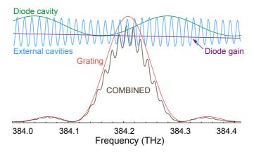
**Figure 1.4:** Schematic representation for the various frequency-dependent factors of an ECDL, adapted from Ref. [1], for wavelength  $\lambda=780\,\mathrm{nm}$  and external cavity length  $L_{\mathrm{ext}}=15\,\mathrm{mm}$ .
