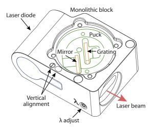
**Figure 1.1:** Sketch of MOGLabs LDL monolithic block external cavity diode laser.
