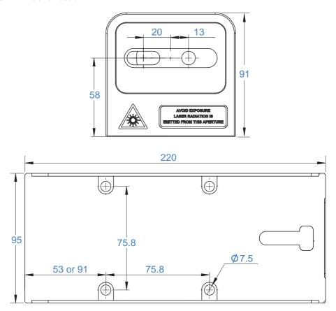
Figure A.3: Dimensions of CEF laser head.
